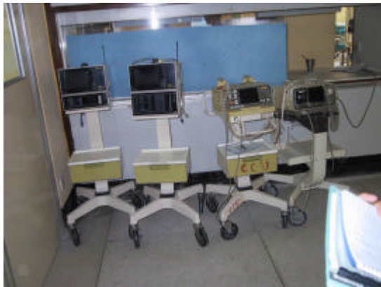
ECG monitors on rollers with potential risk of sliding and overturning.
