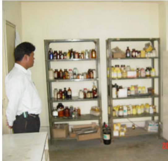
Chemical and medicine bottles on shelves pose a risk of falling.
